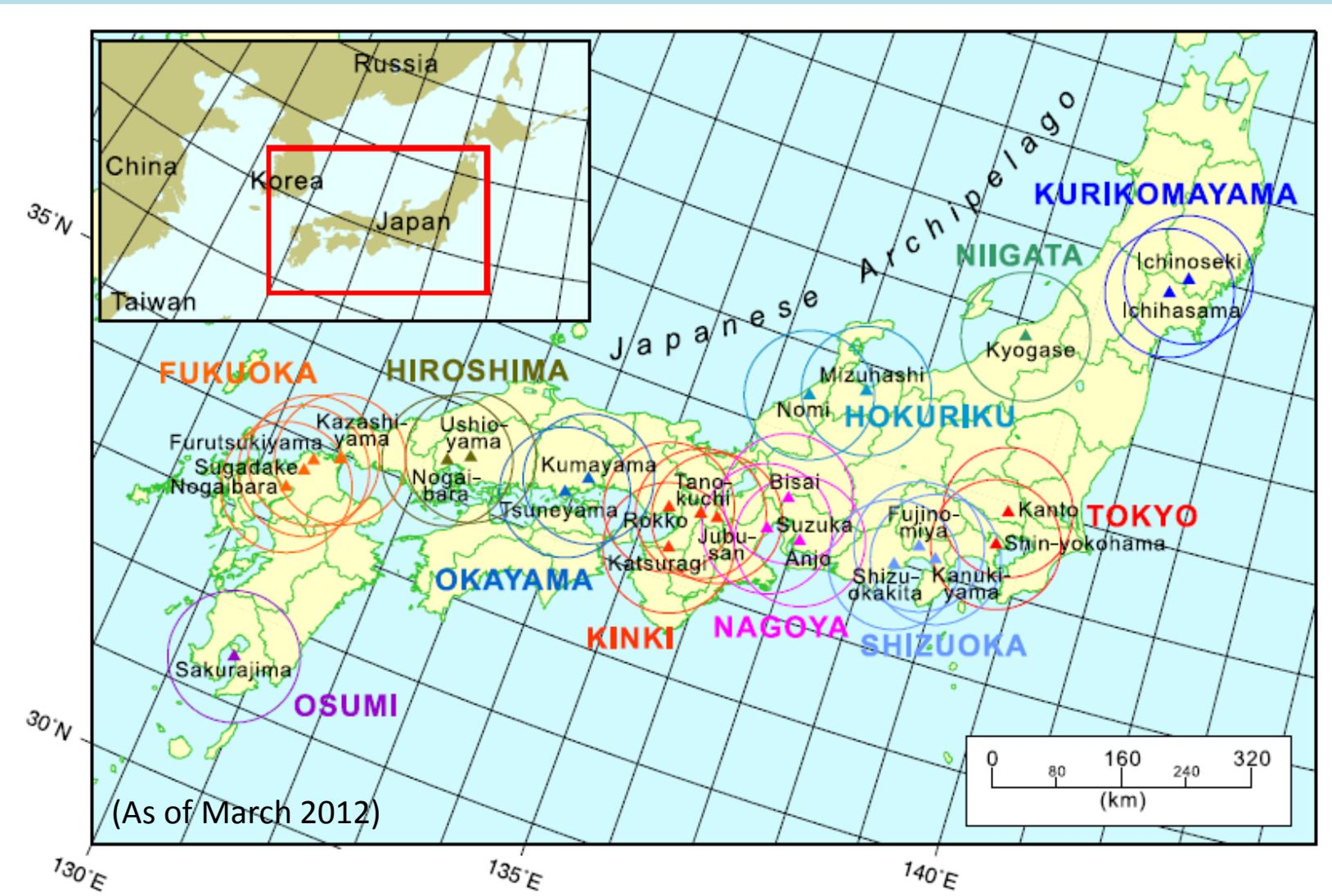
The Ministry of Land, Infrastructure, Transport and Tourism (MLIT) started to construct X-band polarimetric radar network in 2009 to monitor heavy rainfall in urban areas. A total of 27 (35) radars are operating in 2012 (2013).
