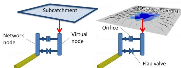
**Figure 2.** Hypothetical connections of sub-catchments (left) and surface overland (right) with the sewer network used in the model to better model flooding mechanism.
