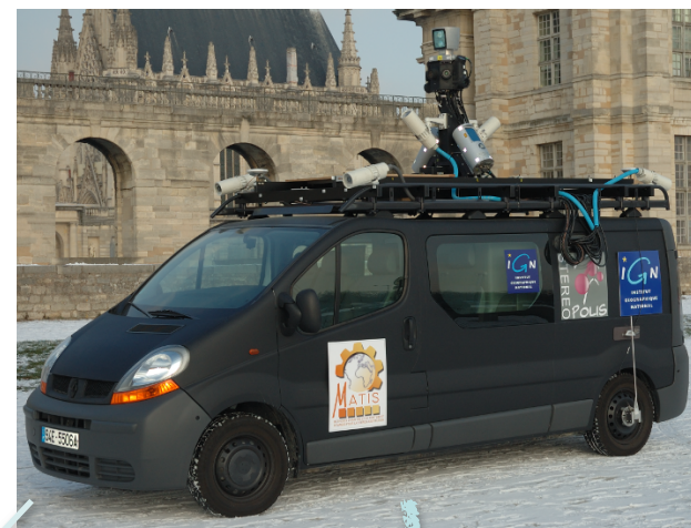
IGN STEREOPOLIS II mobile mapping system
