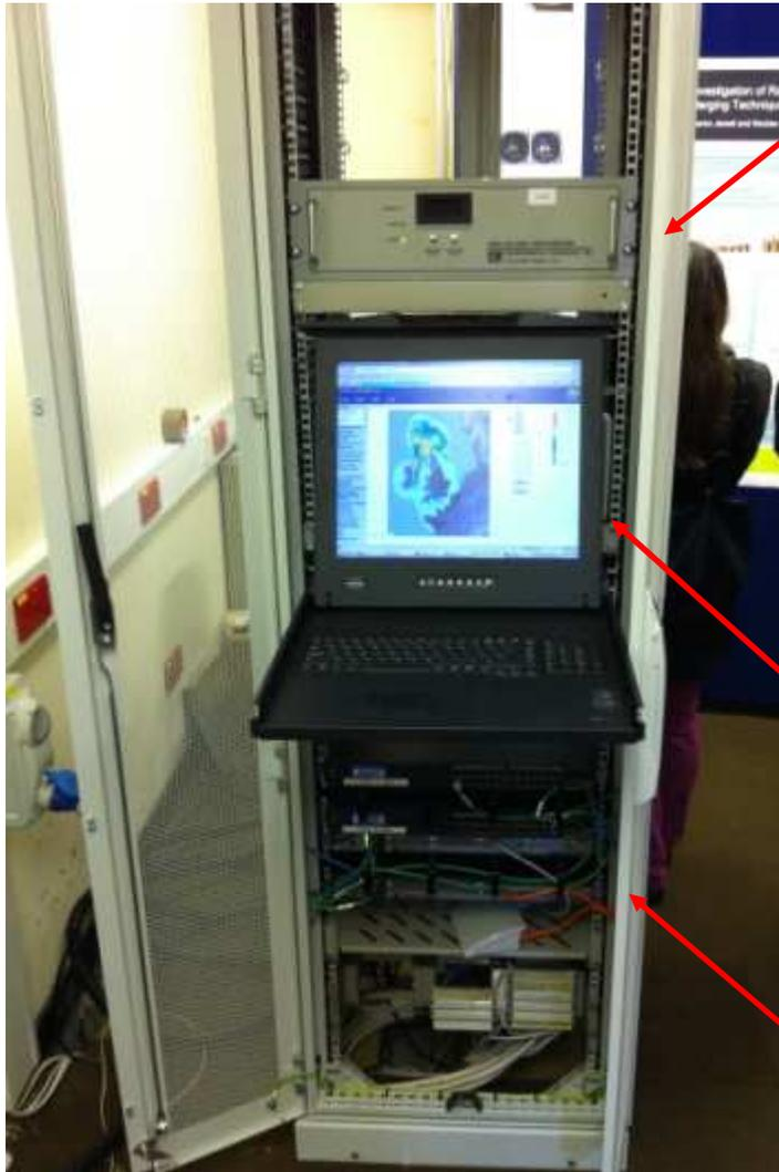
**Pump to inject air in the wave guide to keep it dry**
