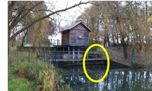
Figure 10: Water depth sensor of "Bassin des Bas-Près"
