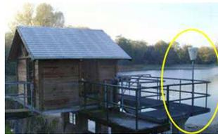
Figure 9: Rain gauge (circled) located near a house used for remote control of a storage basin.
