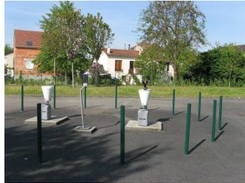
Figure 8: Rain gauges located near the Gérard Philippe basin
