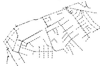
Figure 12: Modelled sewer network for the Kodak catchment
