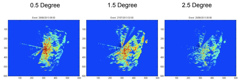
Dry weather images at each antenna elevation
