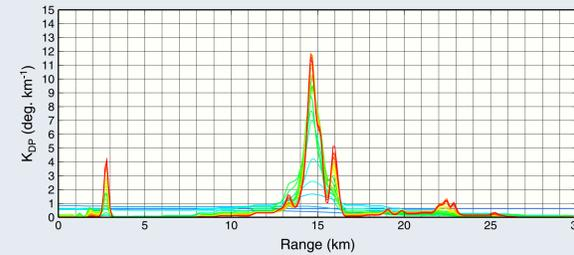
$K_{DP}$  profile modifications at each BFGS iteration step. Colors of the profiles correspond to the color plots shown in upper right.
