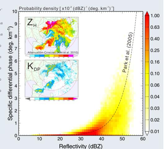
Probability density of scatter plots of  $Z_h$  versus  $K_{DP}$  calculated by this method ( $C_{lpf} = 1 \times 10^{10}$ ). The data are observed by NIED's X-band dual-pol. radar at 1402 UTC 9 July 2005.
