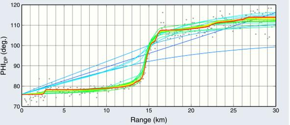
$\Phi_{DP}$  profile modifications at each BFGS iteration step. Colors of the profiles correspond to the color plots shown in upper right.
