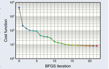
An example of the minimizing of the cost function by BFGS method. Colors of plots correspond to the colors of  $K_{DP}$  and  $\Phi_{DP}$  profiles shown below.
