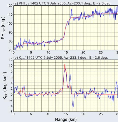
a) The range profiles of the differential phase. Blue profile is observed by NIED's X-band dual-polarimetric radar at Ebina, Japan, at 1402 UTC 9 July 2005. The range gate width of this radar is 100 m. Red profile is analyzed from the observed data by this method ( $C_{lpf} = 1 \times 10^{10}$ ).
