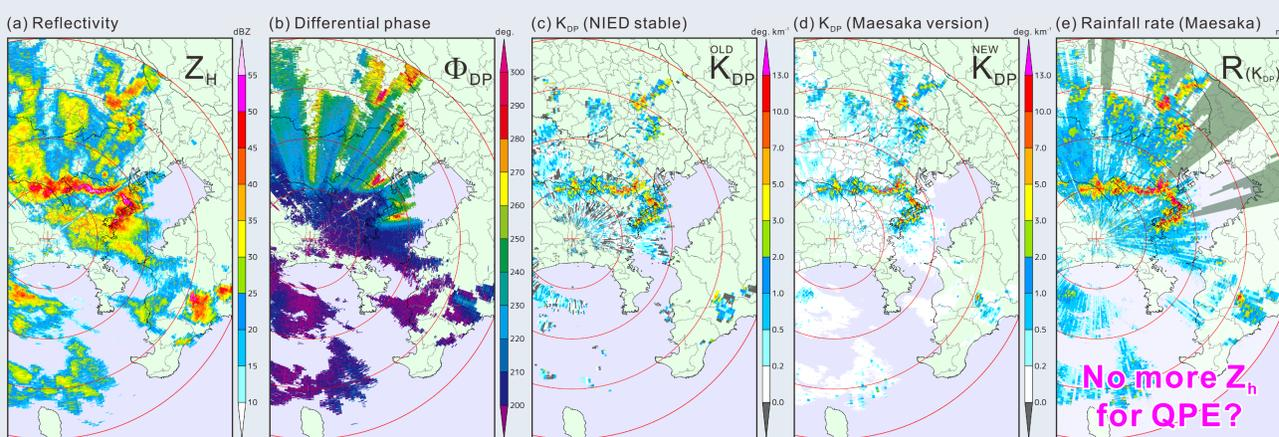
PPI images of NIED's X-band polarimetric radar at Ebina city at 0500 UTC 10 May 2012. The elevation angle is 1.2. Range circles are drawn at 20 km intervals from the radar. a) Observed reflectivity (no attenuation correction), b) Observed differential phase, c) Specific differential phase estimated by classic method (NIED stable algorithm: the
