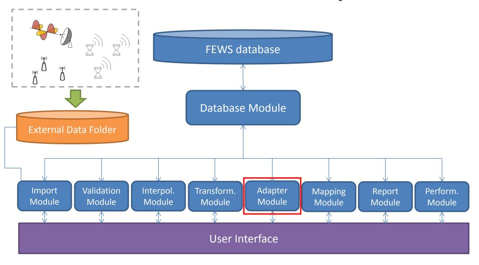
As can be seen, it has a central database to which a number of modules with different functionalities can be plugged. One of these modules is the "Adapter", which enables linking external models to the system (e.g. algorithms for rainfall nowcasting and downscaling, hydraulic models, amongst others).
