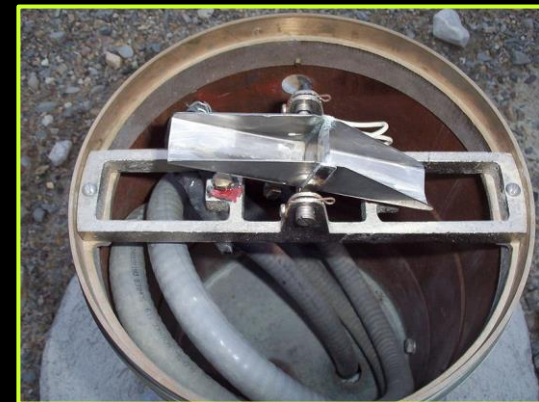
Tipping Bucket Raingauge mechanism
