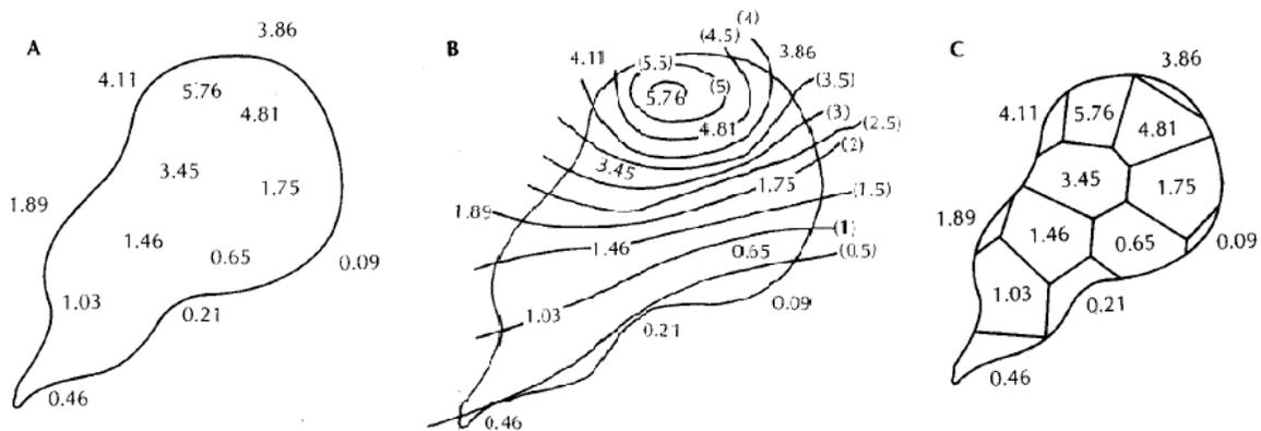
Figure 25: Rainfall interpolation methods based on gauges: A: a drainage basin with rain gauges (their position is marked by their respective measurement values), B: the spatial rainfall distribution based on the isohyetal method and C: the spatial rainfall distribution based on the Thiessen method (adapted from Fetter, 1994)
