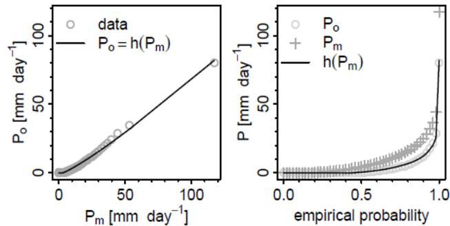
Figure 18: Example of the Quantile mapping method: left: a quantile quantile (QQ-) plot of observed ( $P_o$ ) and modeled ( $P_m$ ) precipitation and a transformation function ( $h$ ) to map the quantiles together, right: the empirical cumulative distribution function (CDF) of the observed modeled and transformed ( $h[P_m]$ ) precipitation (after Gudmundsson et al., 2012).
