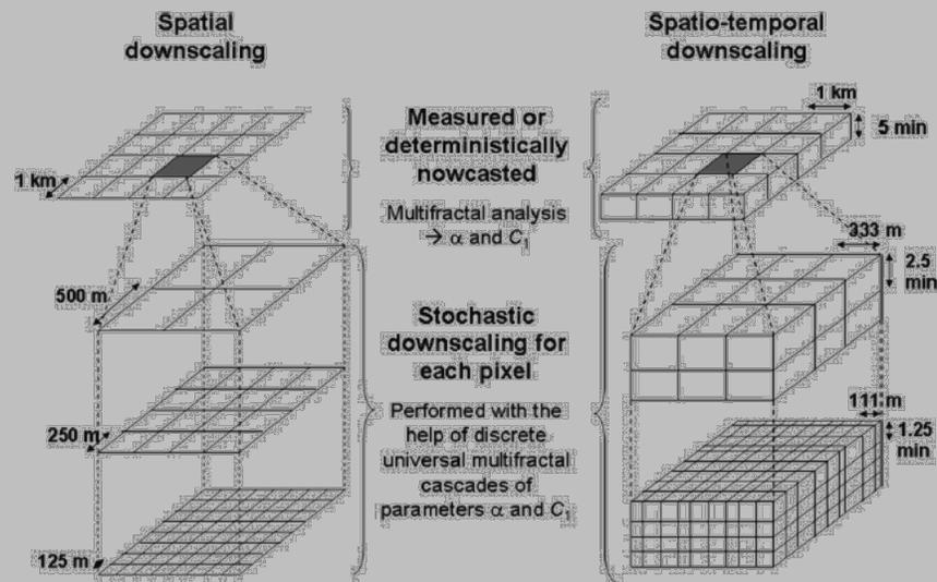
Figure 15: Illustration of the spatial (left) and spatio-temporal (right) downscaling techniques
