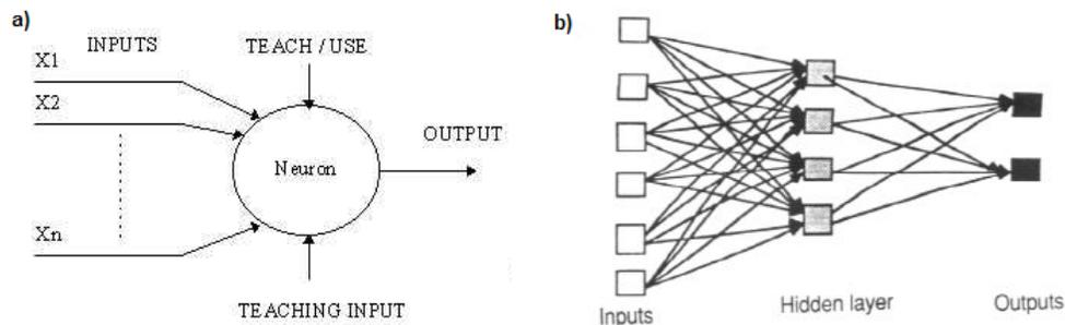
Figure 19: Artificial neural network schematization: a) representation of one single neuron and b) representation of a simple feed-forward neural network architecture (adapted from Stergiou and Siganos, 1997)
