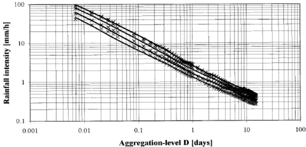
Figure 21: IDF-relationships for return periods of 27, 9, 2.7 and 1 years; comparison of calibrated IDF-relationships (full lines) with observations (source: Willems, 2000)
