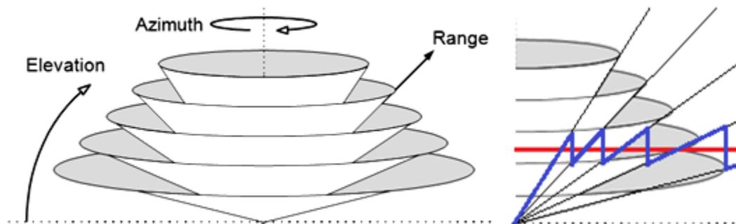
Figure 9: a) Radar scanning strategy: example of scans at different elevation levels (adapted from EG-CLIMET MediaWiki)
