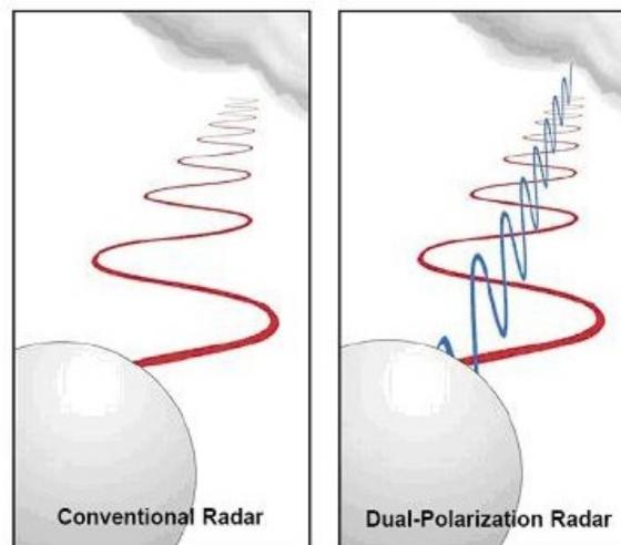
Figure 2: Working principle of a conventional (single, horizontal polarization) radar versus a dual polarization (horizontal and vertical) radar (Source: NOAA)
