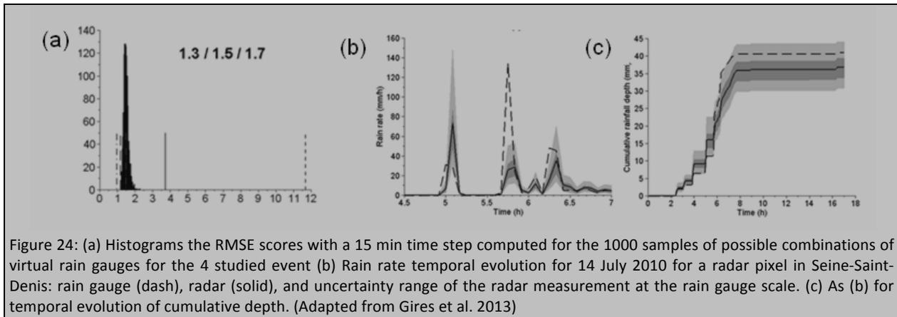
Figure 24: (a) Histograms the RMSE scores with a 15 min time step computed for the 1000 samples of possible combinations of virtual rain gauges for the 4 studied event (b) Rain rate temporal evolution for 14 July 2010 for a radar pixel in Seine-Saint-Denis: rain gauge (dash), radar (solid), and uncertainty range of the radar measurement at the rain gauge scale. (c) As (b) for temporal evolution of cumulative depth. (Adapted from Gires et al. 2013)
