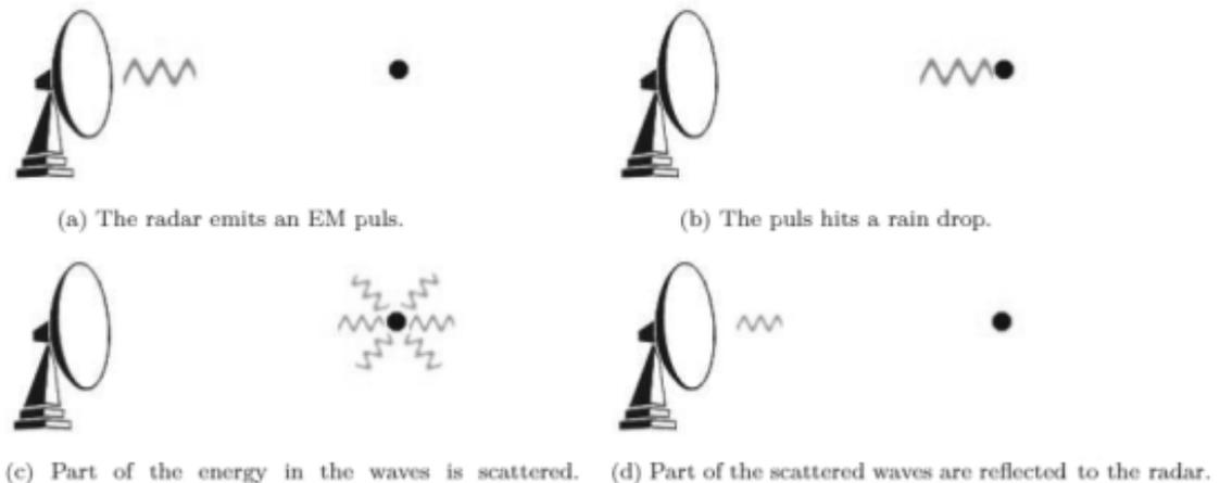
Figure 1: Working principle of a weather radar (after Cain, 2002)
