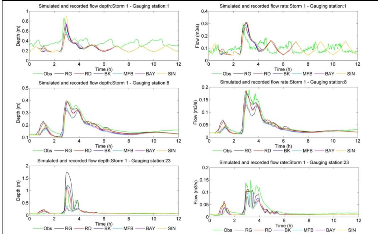
Figure 7: Comparisons of observed and simulated flow depth (left) and flow rate (right) hydrographs of Portobello’s Storm 1 at three gauge stations selected from different part of the catchment (the points FM1, FM8 and FM23 in Figure 3(b)): gauge 1 (top), gauge 8 (middle) and gauge 23 (bottom).
