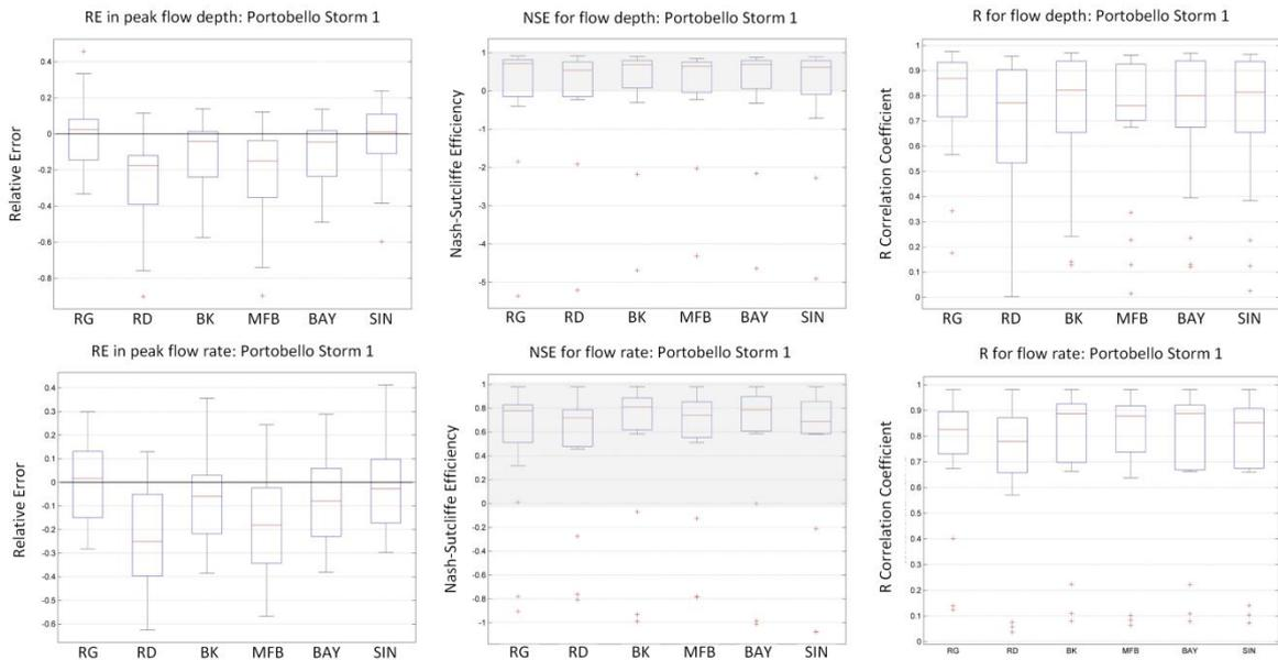
Figure 8: Boxplots of  $RE$  (left),  $NSE$  (middle) and  $R$  (right) for flow depths and rates simulated using different rainfall inputs for Portobello’s Storm 1. The shaded areas in the  $NSE$  boxplots correspond to the region of positive  $NSE$  values ( $0 < NSE < 1$ ).
