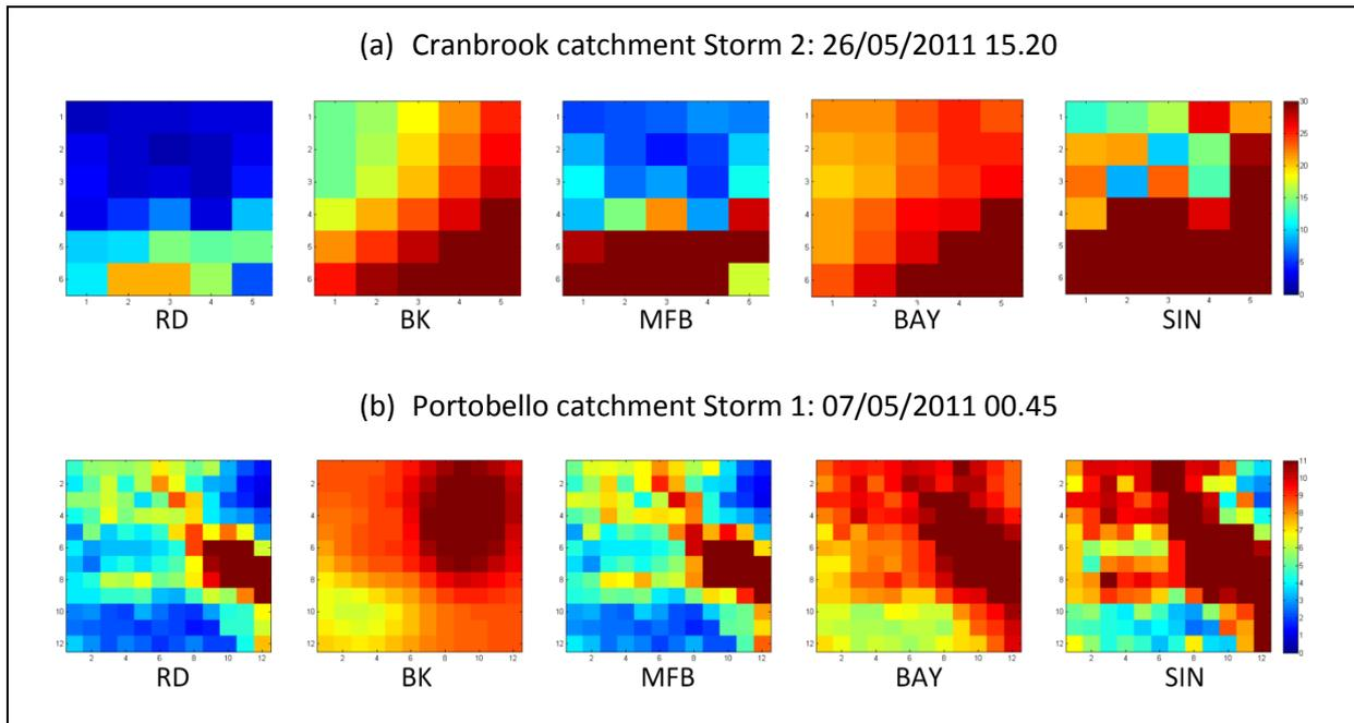
Figure 4: Images of RD, BK and adjusted rainfall estimates at peak intensity times of (a) Cranbrook's Storm 2 and (b) Portobello's Storm 1.
