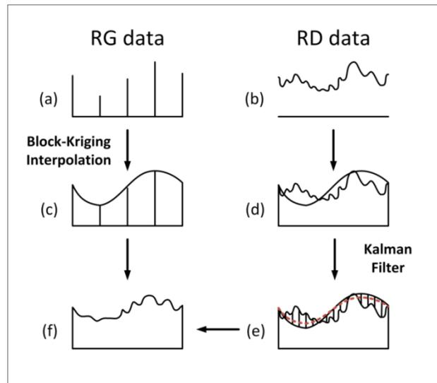
Figure 1: Schematic of Bayesian radar-raingauge data merging (Todini, 2001). This figure was adapted from Figure 3 of Ehret et al. (2008).
