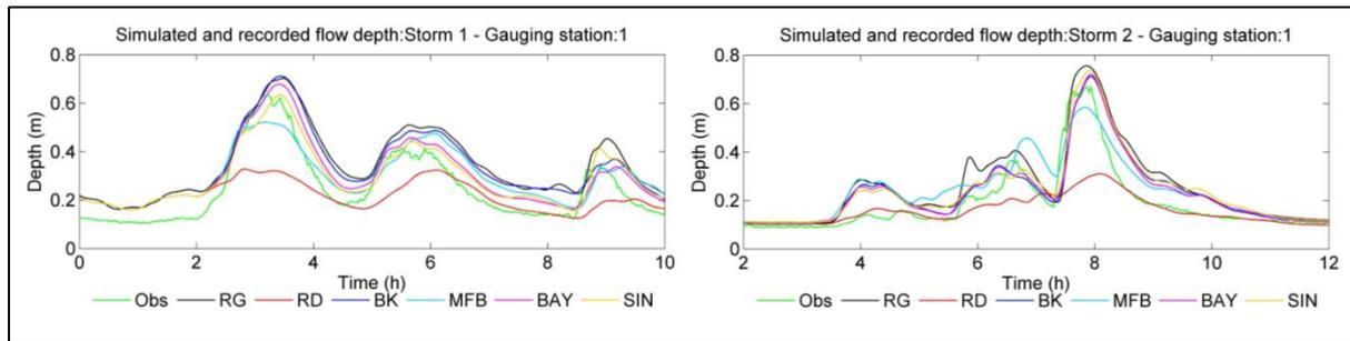
Figure 6: Comparison of observed and simulated flow depth hydrographs for different rainfall inputs at the Valentine sewer (Point A in Figure 2(b)) in the Cranbrook catchment: (left) Storm 1 and (right) Storm 2.
