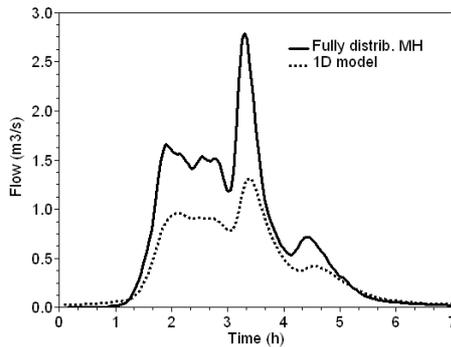
Figure 5: Comparison of simulated flow at the outlet for both models
