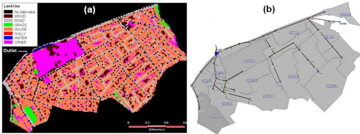
Figure 4: (a) Map of the land use distribution with a 10 m resolution used in Multi-Hydro. The sewer network modelled with SWMM is superposed to this map (the nodes, which are either a manhole or a gully, and conduits are visible along most of the roads). (b) Snapshot of the representation of this area with the 1D model Canoe. The sub-catchments and the modelled sewer network are visible.
