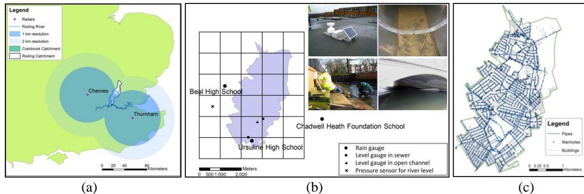
Figure 1. Cranbrook catchment (a) location of the catchment in relation to radars and the Roding River catchment; (b) monitoring system; (c) sewer network
