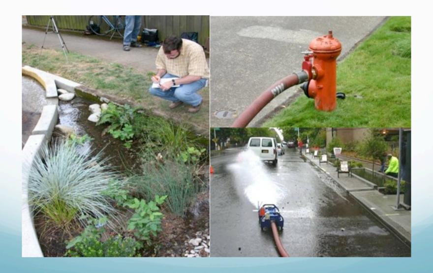
Additional green elements at street level may reduce run-off peaks in sewer systems (after a test that is shown on the pictures on the right)
