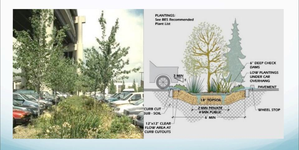
Blue-green solution at parking lots to avoid stormwater problems (the design is on the right and the final result is on the left)
